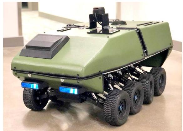
FIGURE 3. The Scaled Electric Combat Vehicle Prototype
